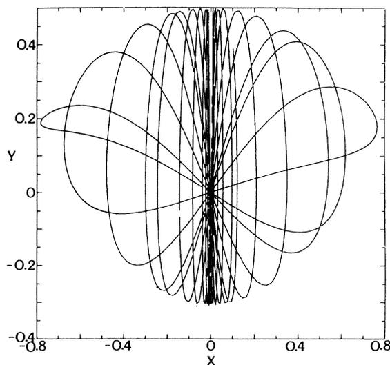
FIG. 1. The  $x$ - $y$  trajectory of the generalized Hénon-Heiles system, (2.1) and (2.2b), for  $A=1$ ,  $B=4$ ,  $C=-1$ , and  $D=6$ , and for the initial values  $x(0)=0.01$ ,  $y(0)=0.5$ ,  $\dot{x}(0)=\dot{y}(0)=0$ .
