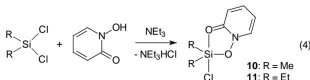
The X-ray structure of **10** reveals a distorted TBP coordination sphere (Figure 10). Deviation from a regular TBP polyhedron is seen in the apical O–Si–Cl angle of 167.52(3)° and in the sum
